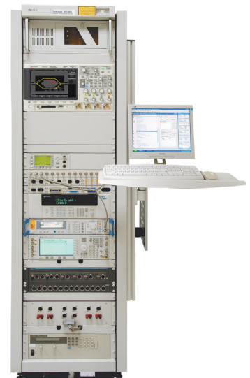
Figure 27. Automated test rack
